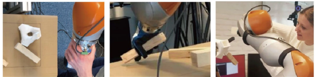
Figure 2. CV and HRI assembly of scaled prototype. Robots equipped with CV recognize and manipulate irregular timber blocks ( left ) and ( center ), while the ( right ) image shows collaborative task-sharing with a researcher. © TU Delft [27].
