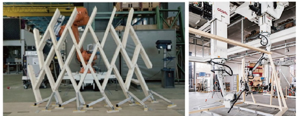
Figure 1. Robotically assembled prototypes using one or more robots: precise robotic placement of short, interlocking timber elements into a diamond grid ( left ) and gantry-based system ( right ). © ETH Zurich [23].
